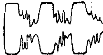
SSB SIGNAL, VOICE INPUT. SQUARING AUDIO PEAKS. EXCESSIVE SPEECH GAIN
