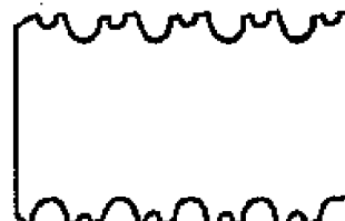
SSB SIGNAL, TONE INPUT BALANCED MOD DETUNED (L3)
