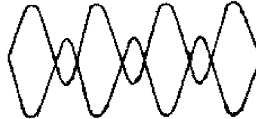
DRC DOUBLE SIDEBAND REDUCED CARRIER OBTAINED BY REDUCING CARRIER LEVEL AND INCREASING AUDIO INPUT LEVEL.
