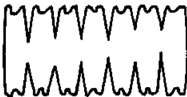
SSB SIGNAL, TONE INPUT INSUFFICIENT 9000 kc. XTAL OSCILLATOR OUTPUT
